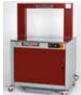
HCSM2000 Automatic 50 Cycles / minute
